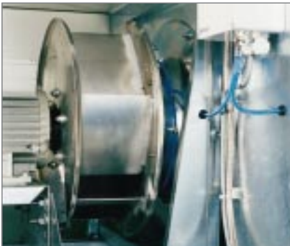
Ringleitung an der Ventilator-Trennwand Closed circuit on the ventilator partition
